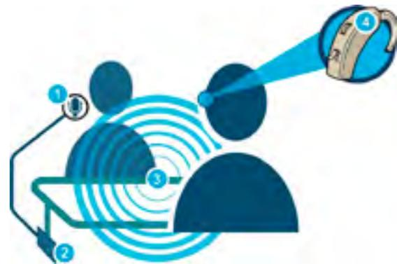
These systems are designed for one-to-one use and are normally found at service tills, bank counters (where glazed security screens are used the loop is often provided in conjunction with a duplex intercom system), reception desks and checkouts.
